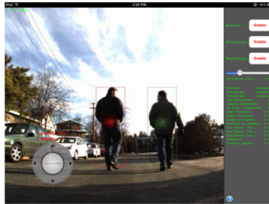
Figure 13: In-situ sensing, tracking pedestrians
