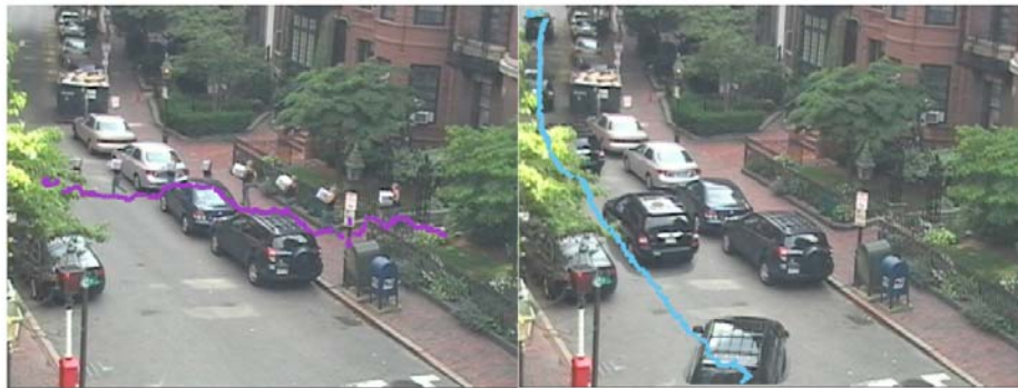
Figure 14: Using video to track vehicles and pedestrians on the same backdrop
