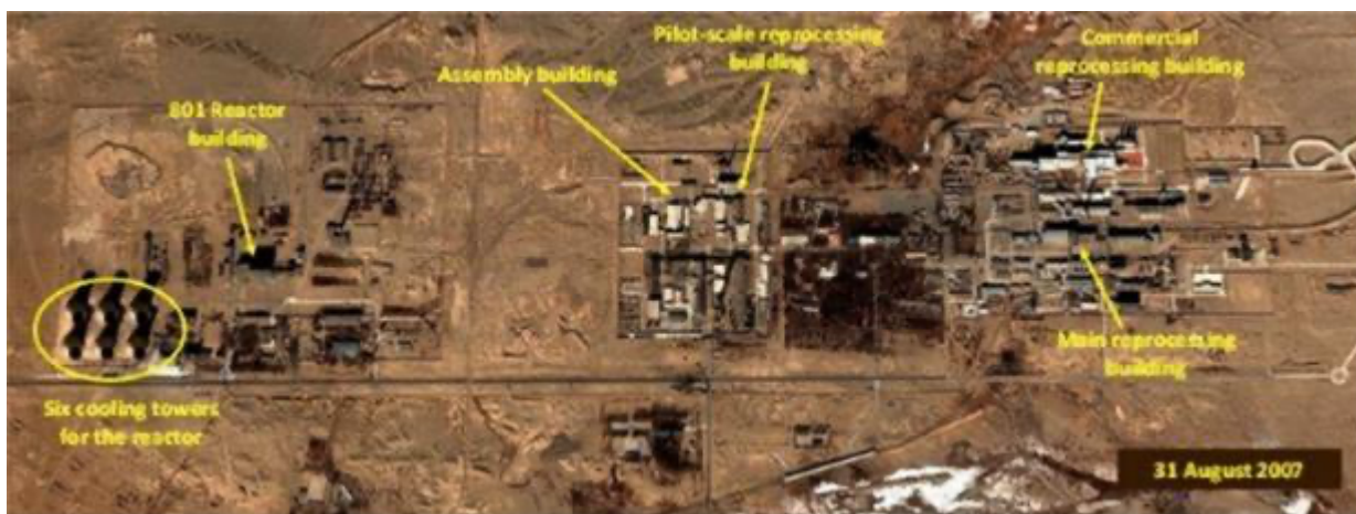
Figure 5. Detail of the 404 Plant reactor and reprocessing area. The Assembly building is the one in which the original nuclear weapon parts were prepared for China’s first nuclear test.
