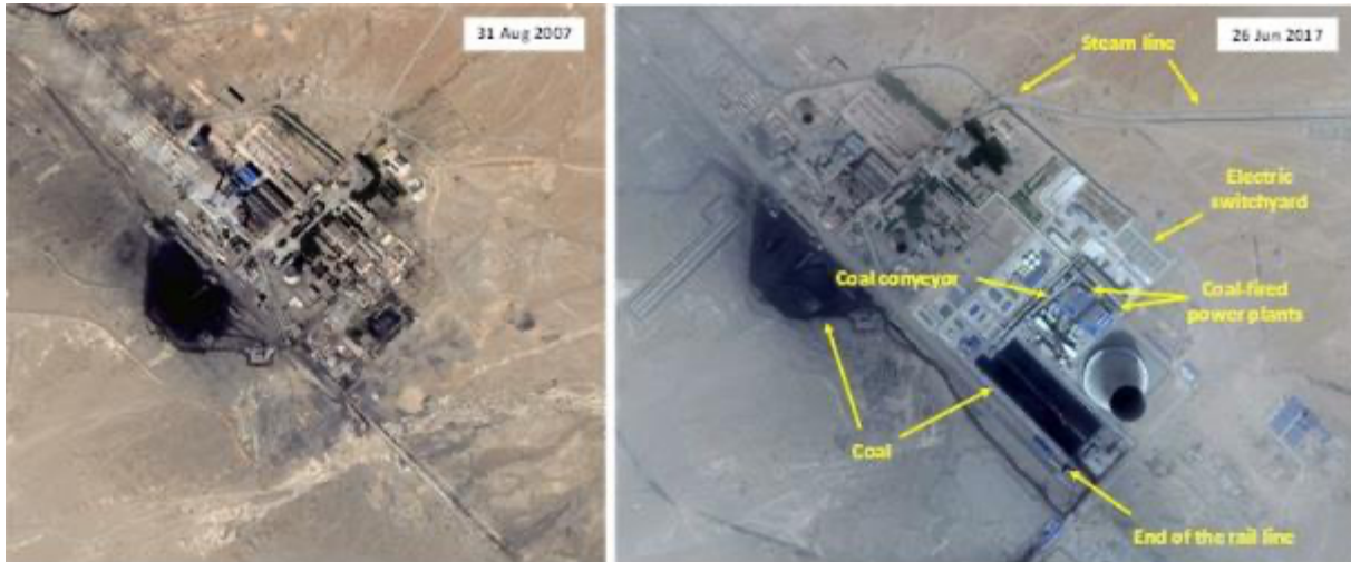
Figure 11. Expansion of the coal-fired electrical generation capacity at the 404 Plant site, in an area near the reactor and reprocessing area. One can see that the new cooling tower is much larger than the existing cooling towers in the area. The smaller cooling towers are comparable in size to the six cooling towers used by the reactor.
